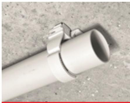
For mounting conduits on concrete and drywall the FC Flexi-Clip™ is connected to the ESD-System, for mounting on cable trays it is connected to the EDV or ESV. The FC Flexi-Clip™ can also be fastened by using a screw.
