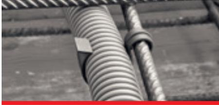
The conduit is pushed into the big opening, with the small opening attached to the wire. Fixings in the small opening prevent the clip from sliding.
